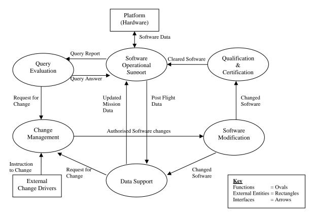
Figure 5 - Software and Data Support Model
