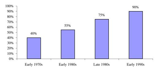
Figure 6 - Increase in Through-life Software Maintenance Cost
